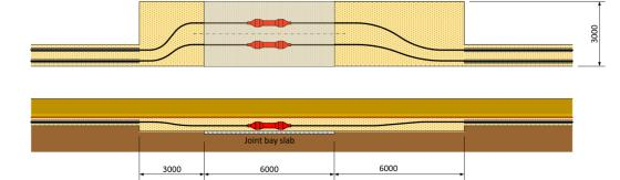
Typical joint-bay dimensions for 1 x 320 kW HVDC circuit. Additional room must be provided in front and behind each joint-bay location to adequately accommodate cable drums and pulling equipment.
